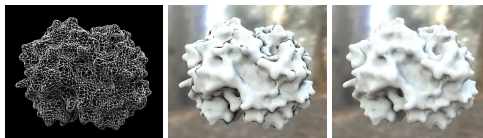
Figure 4: Vertex filtering optimization for the computation of M has to be done carefully, otherwise artifacts will occur (middle). Left: wireframe; right: correct rendering.
