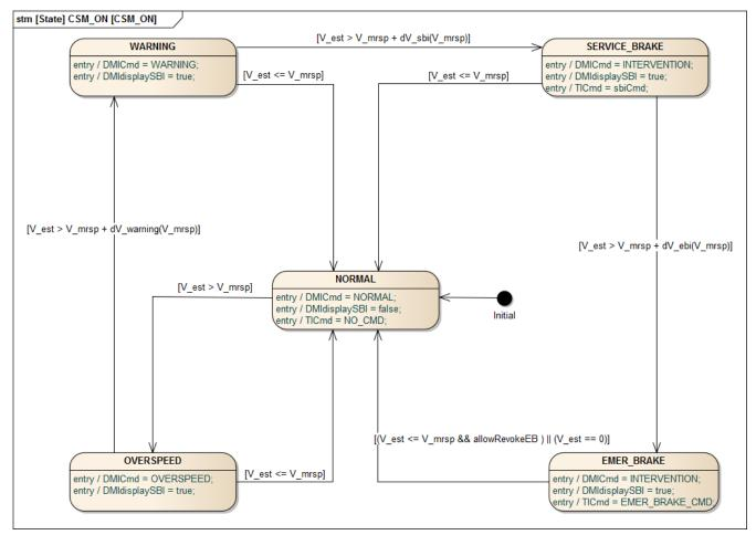
Figure 5. Ceiling speed monitoring state machine.
