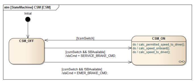
Figure 4. Ceiling speed monitoring – top-level state machine.
