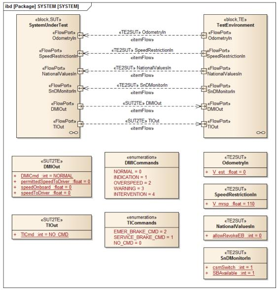
Figure 1. System interface of the ceiling speed monitor.
