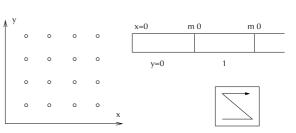
Figure 13: Volume data layout should match the order of traversal of the octree.
