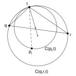
Figure 44: If triangle T(q, r, t) is in conflict with  $p_i$  then former Delaunay edge  $\overline{qr}$  must be replaced by  $\overline{p_i t}$ .
