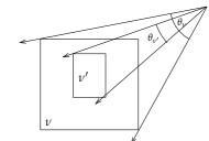
Figure 38: The probability of a ray hitting a child box can be extimated by the surface area.
