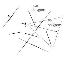
Figure 25: BSP trees are an efficient data structure encoding visibility order of a set of polygons.
