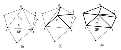
Figure 45: Updating  $DT_{i-1}$  after inserting the new site  $p_i$ . In (ii) the new Delaunay edges connecting  $p_i$  to q, r, s have been added, and edge  $\overline{qr}$  has already been flipped. Two more flips are necessary before the final state shown in (iii) is reached.
