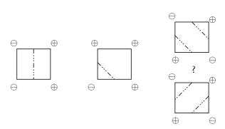
Figure 11: Cells straddling the isosurface are triangulated according to a lookup table. In some cases, several triangulations are possible, which must be resolved by heuristics.
