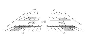
Figure 53: Using an image pyramid, the texture synthesis process becomes fairly robust against different scales of detail in the sample images.
