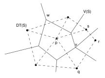
Figure 43: Voronoi diagram and Delaunay triangulation.
