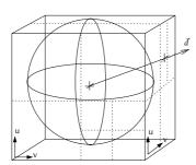
Figure 19: With the direction cube, we can discretize directions, and organize them with any hierarchical partitioning scheme.
