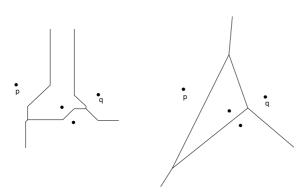
Figure 46: The Voronoi diagram of a point set in  $L_1$  and  $L_2$ . Note, that there are structural differences.
