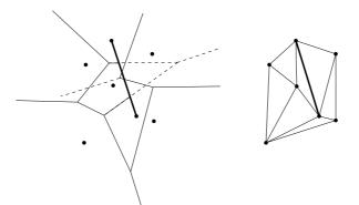
Figure 49: The constrained Voronoi diagram VD(S, L) and its dual.
