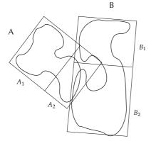
Figure 41: Hierarchical collision detection can discard many pairs of polygons with one BV check. Here, all pairs of polygons in  $A_1$  and  $B_2$  can be discarded.
