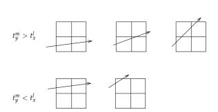
Figure 17: The sub-cell that must be traversed first can be found by simple comparisons. Here, only the case  $t_x^l > t_y^l$  is depicted.
