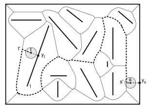
Figure 51: Computing a collision-free path from *s* to *t* for a circle-shaped robot in the presence of polygonal obstacles.
