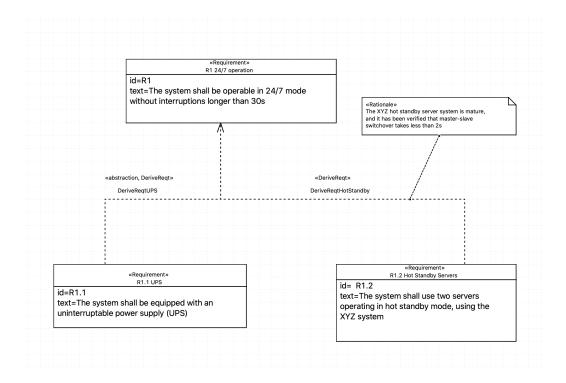
Figure 4.1: Example of supplier requirement and two derived requirements.
