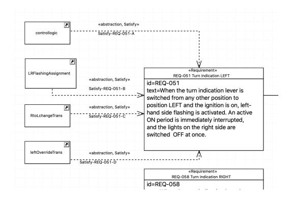
Figure 3.5: Tracing a behavioural requirement to parts, transitions, and opaque behaviours.
