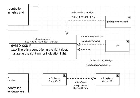
Figure 3.3: Tracing a requirement to parts and flows.
