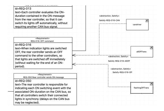
Figure 3.4: Tracing a behavioural requirement to parts and transitions.
